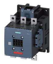
power contactor, AC-3e/AC-3 265 A, 132 kW / 400 V AC (50-60 Hz) / DC Uc: 200-277 V PLC input 24 V DC 3-pole, auxiliary contacts 2 NO + 2 NC permanently mounted drive: electronic main circuit: busbar control and auxiliary circuit: screw terminal
