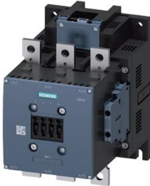
power contactor, AC-3e/AC-3 265 A, 132 kW / 400 V AC (50-60 Hz) / DC U<sub>c</sub>: 21-27.3 V PLC input 24 V DC 3-pole, auxiliary contacts 2 NO + 2 NC drive: electronic main circuit: busbar control and auxiliary circuit: screw terminal
