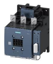
power contactor, AC-3e/AC-3 225 A, 110 kW / 400 V AC (50-60 Hz) / DC Uc: 200-277 V PLC input 24 V DC 3-pole, auxiliary contacts 1 NO + 1 NC drive: electronic main circuit: busbar control and auxiliary circuit: screw terminal with remaining lifetime indicator
