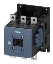
power contactor, AC-3e/AC-3 225 A, 110 kW / 400 V without operating mechanism 3-pole, auxiliary contacts 2 NO + 2 NC main circuit: busbar control and auxiliary circuit: screw terminal
