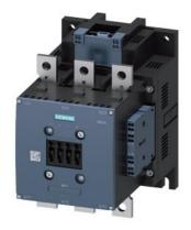
power contactor, AC-3e/AC-3 225 A, 110 kW / 400 V AC (50-60 Hz) / DC Uc: 21-27, 3 V PLC input 24 V DC 3-pole, auxiliary contacts 2 NO + 2 NC drive: electronic main circuit: busbar control and auxiliary circuit: spring-loaded terminal
