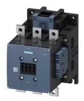
power contactor, AC-3e/AC-3 225 A, 110 kW / 400 V AC (50-60 Hz) / DC Uc: 200-220 V 3-pole, auxiliary contacts 2 NO + 2 NC drive: conventional main circuit: busbar control and auxiliary circuit: spring-loaded terminal
