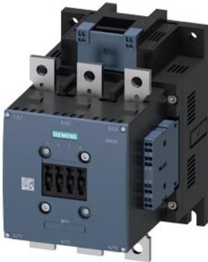
power contactor, AC-3e/AC-3 225 A, 110 kW / 400 V AC (50-60 Hz) / DC Uc: 23-26 V 3-pole, auxiliary contacts 2 NO + 2 NC drive: conventional main circuit: busbar control and auxiliary circuit: spring-loaded terminal
