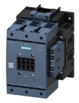
power contactor, AC-3e/AC-3 185 A, 90 kW / 400 V AC (50-60 Hz) / DC Uc: 23-26 V 3-pole, auxiliary contacts 2 NO + 2 NC drive: conventional main circuit: box terminal control and auxiliary circuit: screw terminal box terminal up to 70  $\,\mathrm{mm^2}$
