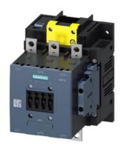
power contactor, AC-3e/AC-3 185 A, 90 kW / 400 V AC (50-60 Hz) / DC Uc: 96-127 V x (0.8-1.1) F-PLC input 24 V DC 3-pole, auxiliary contacts 2 NO + 2 NC drive: electronic main circuit: busbar control and auxiliary circuit: screw terminal
