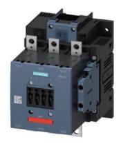
power contactor, AC-3e/AC-3 185 A, 90 kW / 400 V AC (50-60 Hz) / DC Uc: 23-26 V 3-pole, auxiliary contacts 2 NO + 2 NC permanently mounted drive: conventional main circuit: busbar control and auxiliary circuit: screw terminal
