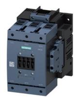
power contactor, AC-3e/AC-3 150 A, 75 kW / 400 V AC (50-60 Hz) / DC Uc: 23-26 V 3-pole, auxiliary contacts 2 NO + 2 NC drive: conventional main circuit: box terminal control and auxiliary circuit: screw terminal box terminal up to 70 mm<sup>2</sup>
