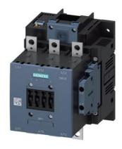
power contactor, AC-3e/AC-3 150 A, 75 kW / 400 V Uc: 24 V DC x (0.7-1.25) PLC input 24-110 V DC 3-pole, auxiliary contacts 2 NO + 2 NC drive: electronic main circuit: busbar control and auxiliary circuit: screw terminal extended rated condition railroad IEC 60077
