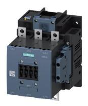
power contactor, AC-3e/AC-3 150 A, 75 kW / 400 V AC (50-60 Hz) / DC Uc: 200-277 V PLC input 24 V DC 3-pole, auxiliary contacts 2 NO + 2 NC drive: electronic main circuit: busbar control and auxiliary circuit: screw terminal
