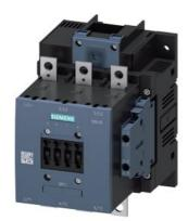
power contactor, AC-3e/AC-3 150 A, 75 kW / 400 V AC (50-60 Hz) / DC Uc: 240-277 V 3-pole, auxiliary contacts 2 NO + 2 NC drive: conventional main circuit: busbar control and auxiliary circuit: screw terminal
