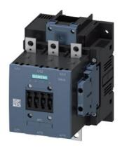
power contactor, AC-3e/AC-3 150 A, 75 kW / 400 V AC (50-60 Hz) / DC Uc: 42-48 V 3-pole, auxiliary contacts 2 NO + 2 NC drive: conventional main circuit: busbar control and auxiliary circuit: screw terminal
