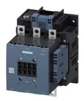
power contactor, AC-3e/AC-3 150 A, 75 kW / 400 V AC (50-60 Hz) / DC Uc: 21-27, 3 V PLC input 24 V DC 3-pole, auxiliary contacts 2 NO + 2 NC drive: electronic main circuit: busbar control and auxiliary circuit: spring-loaded terminal
