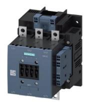
power contactor, AC-3e/AC-3 150 A, 75 kW / 400 V AC (50-60 Hz) / DC Uc: 23-26 V 3-pole, auxiliary contacts 2 NO + 2 NC drive: conventional main circuit: busbar control and auxiliary circuit: spring-loaded terminal
