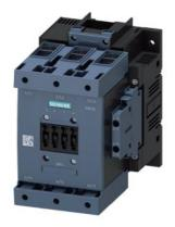
power contactor, AC-3e/AC-3 150 A, 75 kW / 400 V AC (50-60 Hz) / DC Uc: 23-26 V 3-pole, auxiliary contacts 2 NO + 2 NC drive: conventional main circuit: box terminal control and auxiliary circuit: screw terminal
