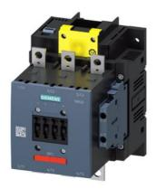
power contactor, AC-3e/AC-3 115 A, 55 kW / 400 V, AC (50-60 Hz) / DC Uc: 96-127 V x (0.8-1.1) F-PLC input 24 V DC 3-pole, auxiliary contacts 2 NO + 2 NC permanently mounted drive: electronic main circuit: busbar control and auxiliary circuit: screw terminal
