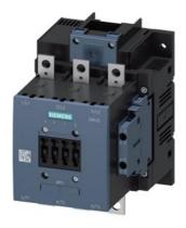
power contactor, AC-3e/AC-3 115 A, 55 kW / 400 V, AC (50-60 Hz) / DC Uc: 240-277 V 3-pole, auxiliary contacts 2 NO + 2 NC drive: conventional main circuit: busbar control and auxiliary circuit: screw terminal
