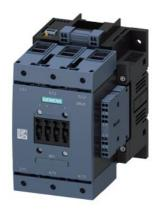
power contactor, AC-3e/AC-3 115 A, 55 kW / 400 V, AC (50-60 Hz) / DC Uc: 96-127 V PLC input 24 V DC 3-pole, auxiliary contacts 2 NO + 2 NC drive: electronic main circuit: box terminal control and auxiliary circuit: spring-loaded terminal
