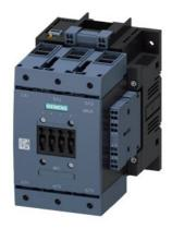
power contactor, AC-3e/AC-3 115 A, 55 kW / 400 V, AC (50-60 Hz) / DC Uc: 21-27.3 V PLC input 24 V DC 3-pole, auxiliary contacts 2 NO + 2 NC drive: electronic main circuit: box terminal control and auxiliary circuit: spring-loaded terminal
