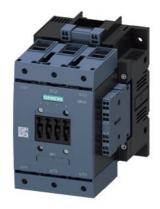
power contactor, AC-3e/AC-3 115 A, 55 kW / 400 V, AC (50-60 Hz) / DC Uc: 200-220 V 3-pole, auxiliary contacts 2 NO + 2 NC drive: conventional main circuit: box terminal control and auxiliary circuit: spring-loaded terminal
