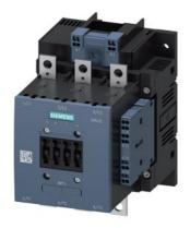
power contactor, AC-3e/AC-3 115 A, 55 kW / 400 V, AC (50-60 Hz) / DC Uc: 220-240 V 3-pole, auxiliary contacts 2 NO + 2 NC drive: conventional main circuit: busbar control and auxiliary circuit: spring-loaded terminal
