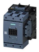
power contactor, AC-3e/AC-3 115 A, 55 kW / 400 V, Uc: 24 V DC x (0.7-1.25) PLC input 24-110 V DC 3-pole, auxiliary contacts 2 NO + 2 NC drive: electronic main circuit: box terminal control and auxiliary circuit: screw terminal
