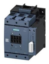
power contactor, AC-3e/AC-3 115 A, 55 kW / 400 V, AC (50-60 Hz) / DC Uc: 200-277 V PLC input 24 V DC 3-pole, auxiliary contacts 1 NO + 1 NC drive: electronic main circuit: box terminal control and auxiliary circuit: screw terminal , remaining lifetime signal
