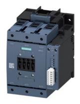
power contactor, AC-3e/AC-3 115 A, 55 kW / 400 V, AC (50-60 Hz) / DC Uc: 96-127 V PLC input 24 V DC 3-pole, auxiliary contacts 1 NO + 1 NC drive: electronic main circuit: box terminal control and auxiliary circuit: screw terminal , remaining lifetime signal
