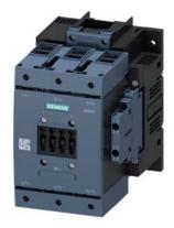
power contactor, AC-3e/AC-3 115 A, 55 kW / 400 V, AC (50-60 Hz) / DC Uc: 200-220 V 3-pole, auxiliary contacts 2 NO + 2 NC drive: conventional main circuit: box terminal control and auxiliary circuit: screw terminal
