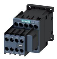
Contactor relay with auxiliary switch 125 V DC Size S00, screw terminal, 4 NC basic unit / EN Varistor plugged on
