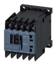
Contactor relay, 4 NO, 100 V AC, 50 Hz, 100 ... 110 V, 60 Hz, Size S00 ring cable lug connection
