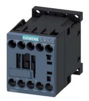
Coupling contactor relay, 4 NO, 24 V DC, 0.7 ... 1.25\* US, with integrated diode, Size S00, screw terminal suitable for PLC outputs
