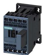
Coupling contactor relay, 3 NO + 1 NC, 24 V DC, 0.85  $\ldots$  1.85\* US, with varistor plugged on, Size S00, Spring-type terminal
