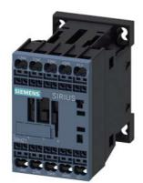
Contactor relay, 3 NO + 1 NC, 24 V DC, integrated varistor Size S00, Spring-type terminal
