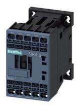
Coupling contactor relay railway 3 NO + 1 NC, 110 V DC, 0.7 ... 1.25\* US, with varistor integrated, Size S00, Spring-type terminal
