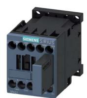
Coupling contactor relay, 3 NO + 1 NC, 24 V DC, 0.85  $\ldots$  1.85\* US, with varistor plugged on, Size S00, screw terminal
