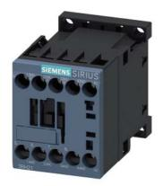
Contactor relay, 3 NO + 1 NC, 480 V AC, 60 Hz, Size S00, screw terminal
