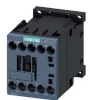
Contactor relay, 3 NO + 1 NC, 208 V AC, 50 / 60 Hz, Size S00, screw terminal
