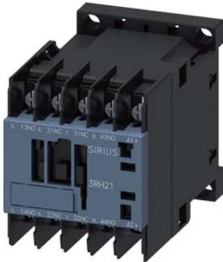
Coupling contactor relay, 2 NO + 2 NC, 24 V DC, 0.7 ... 1.25\* US, with integrated suppressor diode, Size S00, Ring cable lug connection, suitable for PLC outputs
