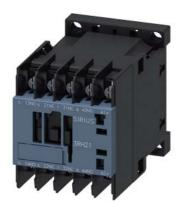
Contactor relay, 2 NO + 2 NC, 24 V DC, Size S00, ring cable lug connection
