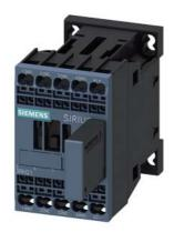
Coupling contactor relay, 2 NO + 2 NC, 24 V DC, 0.85  $\dots$  1.85\* US, with varistor plugged on, Size S00, Spring-type terminal
