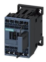
Contactor relay for railway, 2 NO + 1 NC, 110 V DC, 0.7 ... 1.25\* US, with integrated varistor, 3-pole, Size S00, Spring-type terminal for upright mounting position
