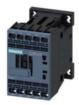
Contactor relay, 2 NO + 2 NC, 42 V AC, 50 / 60 Hz, Size S00, Spring-type terminal
