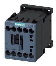
Contactor relay, 2 NC+2 NO 230 V AC, 50/60 Hz Size S00, screw terminal integrated varistor Ambient temperature -30 °C up to 70 °C, thermal rating max. 0.857 Operating range coil 0.95-1.03 US US = 230 V, Tmax 70 °C Frequency of operation 0.857 z
