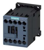
Coupling contactor relay, 2 NO + 2 NC, 24 V DC, 0.7  $\dots$  1.25\* US, with integrated suppressor diode, Size S00, screw terminal suitable for PLC outputs
