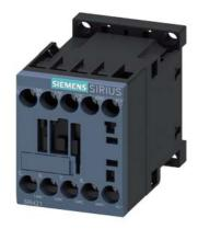
Contactor relay, 2 NO + 2 NC, 24 V DC, with integrated diode, Size S00, screw terminal
