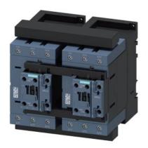
reversing contactor assembly, AC-3e/AC-3, 80 A, 37 kW / 400 V, 3-pole, 20-33 V AC/DC, 50/60 Hz, screw terminal, electrical and mechanical interlock, auxiliary contacts: 2 x 1 NO
