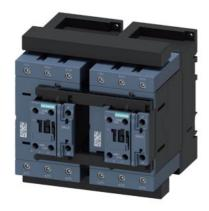
reversing contactor assembly, AC-3e/AC-3, 80 A, 37 kW / 400 V, 3-pole, 110 V AC, 50/60 Hz, screw terminal, electrical and mechanical interlock, auxiliary contacts: 2  $\times$  1 NO
