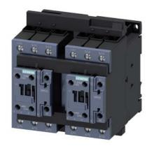
reversing contactor assembly, AC-3e/AC-3, 80 A, 37 kW / 400 V, 3-pole, 20-33 V AC/DC, 50/60 Hz, screw terminal, electrical and mechanical interlock, auxiliary contacts: 2 x 1 NO
