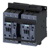
reversing contactor assembly, AC-3e/AC-3, 80 A, 37 kW / 400 V, 3-pole, 230 V AC, 50/60 Hz, screw terminal, electrical and mechanical interlock, auxiliary contacts: 2 x 1 NO
