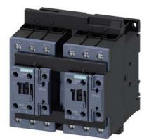
reversing contactor assembly, AC-3e/AC-3, 65 A, 30 kW / 400 V, 3-pole, 110 V AC, 50/60 Hz, screw terminal, electrical and mechanical interlock, auxiliary contacts: 2 x 1 NO
